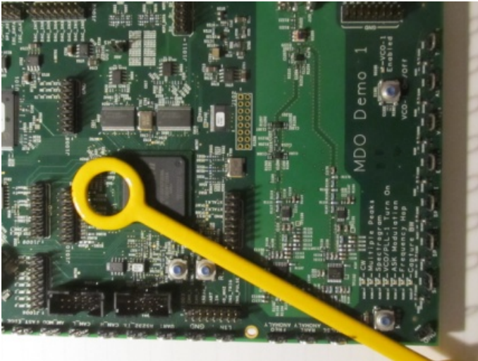
Figure 2: A near-field probe is used to discover the location of the peaks of the offending signal.
